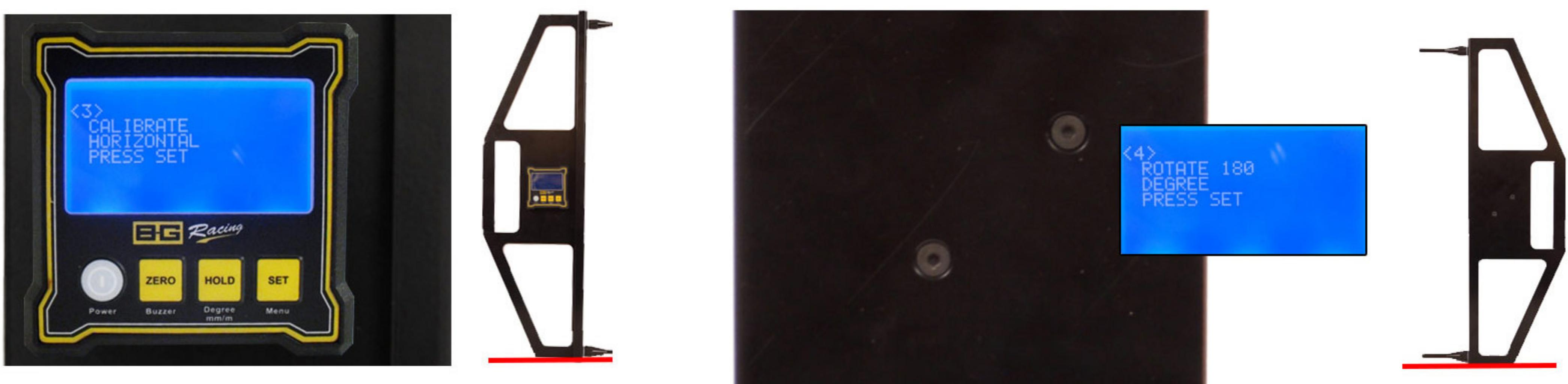
5. Once the buzzer has stopped LCD display "<5> CALIBRATE VERTICAL PRESS SET". Place the pins down onto the flat surface and press the "SET" button again and the buzzer will beep.
