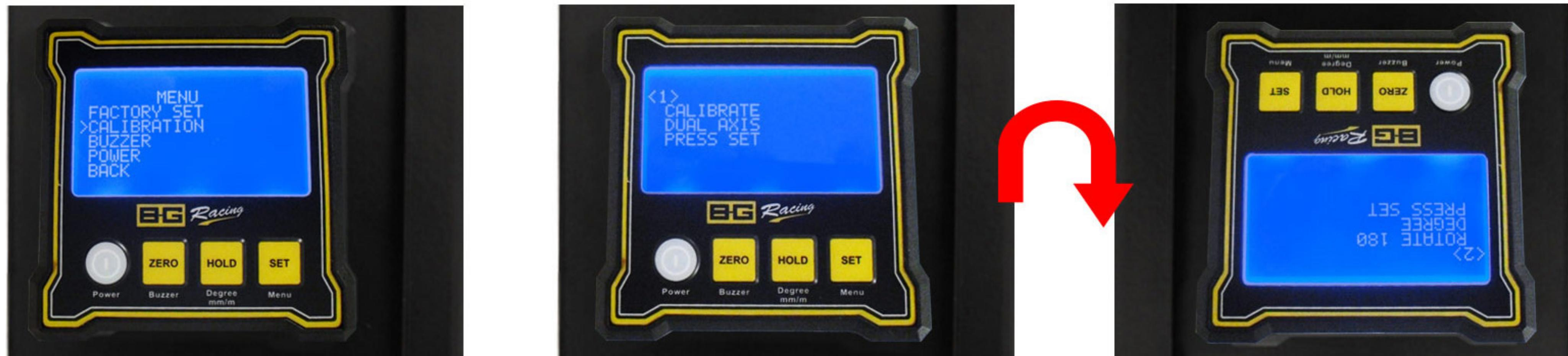
3. Once the buzzer has stopped LCD display "<3> CALIBRATION HORIZONTAL PRESS SET". Stand the frame up so the bottom edge is on the flat surface and press the "SET" button again and the buzzer will beep.
