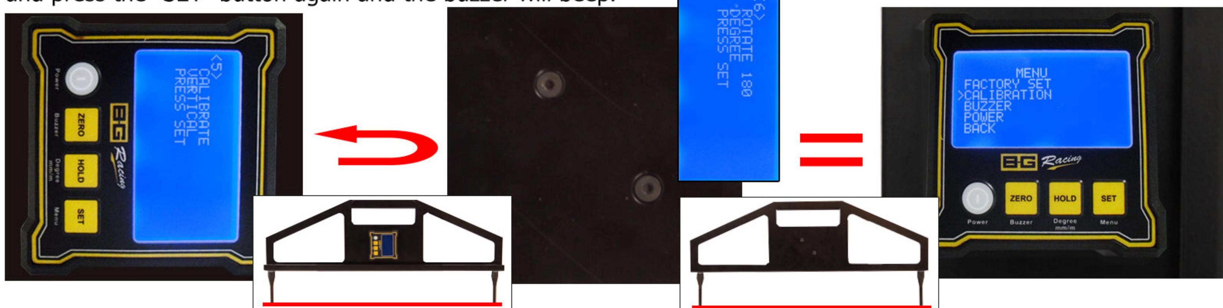
7. The unit is now calibrated, and the unit will display the main menu, using the "ZERO" button & "HOLD" button to toggle, select "BACK" and press "SET" button to return to the measuring display.
